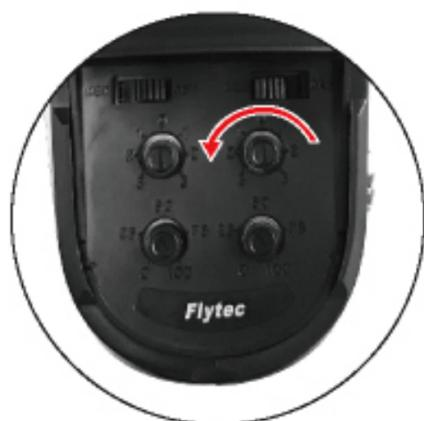
1. Turn the knob to the left to reduce the sensitivity of the throttle knob.
