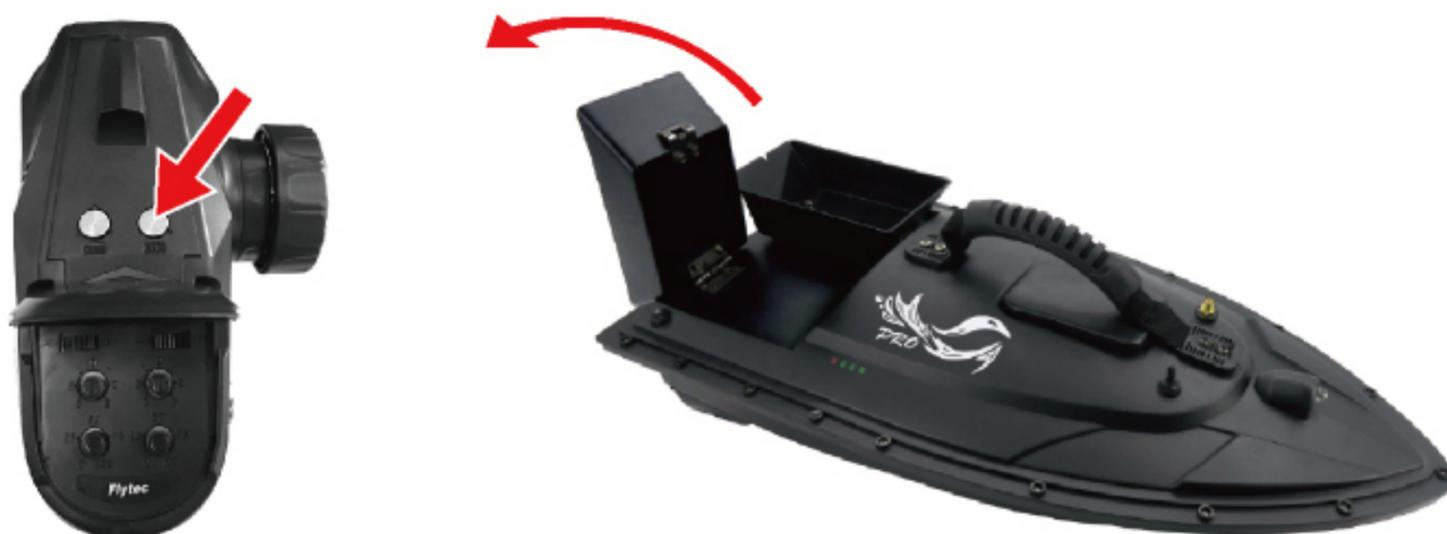
**NOTE:** When you throw the bait, please turn these two buttons to the middle position (as shown on the right, stop the motor working and achieve the silent baiting).
