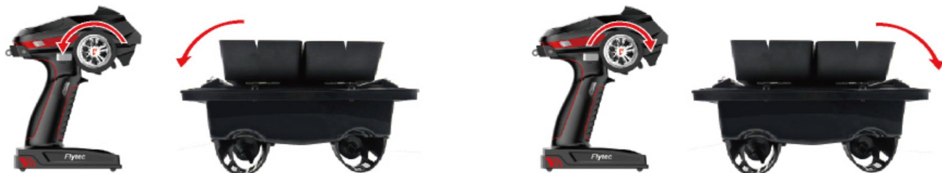
**NOTE:** If you found the above operating direction is opposite to the actual situation, the steering can be switched by pressing "Steering Operation Mode Switch".
