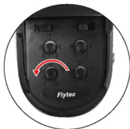
1. Turn the knob to the left to reduce the speed of steering.
